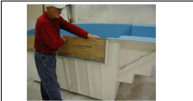
1. All windows are pre-cut for a loose fit. Before removing protective paper, place window in channel to ensure proper fit.
